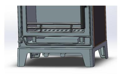
3. Adjust the stove leveling bolts show picture below until the stove is level and evenly supported. Take care not to damage the floor surface.
