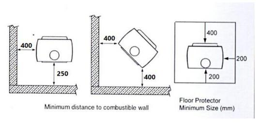
It is recommended that the stove be installed at least 400 mm from combustible materials. However, any household furnishings should be at least 1000mm away as they could be adversely affected by heat.
