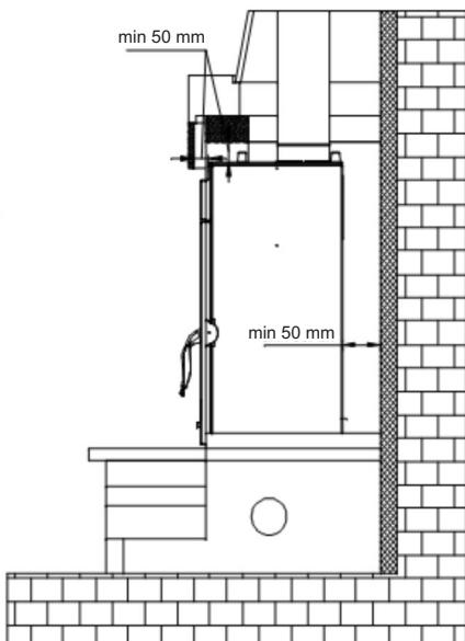
1. Convection air flow is ensured between the enclosed portion of the fireplace and the masonry fireplace wall. To achieve this, minimum distance of 5 cm shall be provided between the 5 cm thick rock wool insulation of the fireplace wall and the insert.
